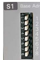
1<sup>st</sup> **Module** address = basic address
