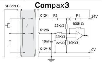
The circuit example is valid for all digital inputs! Signal level:
