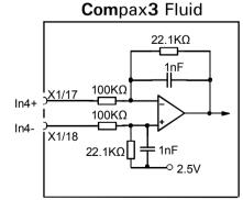
IIN4 and IN5 (X11/19 and X11/20) have the same wiring!
