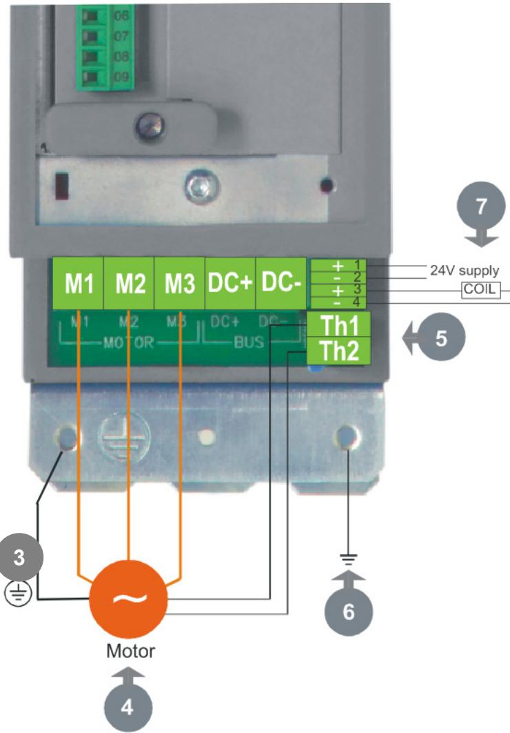
**4** Connect motor leads to M1, M2, M3. Maximum wire sizes:
