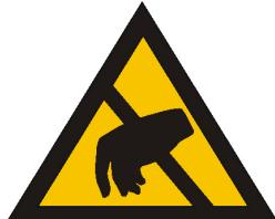
Electrostatic discharge sensitive parts : observe static control precautions.
