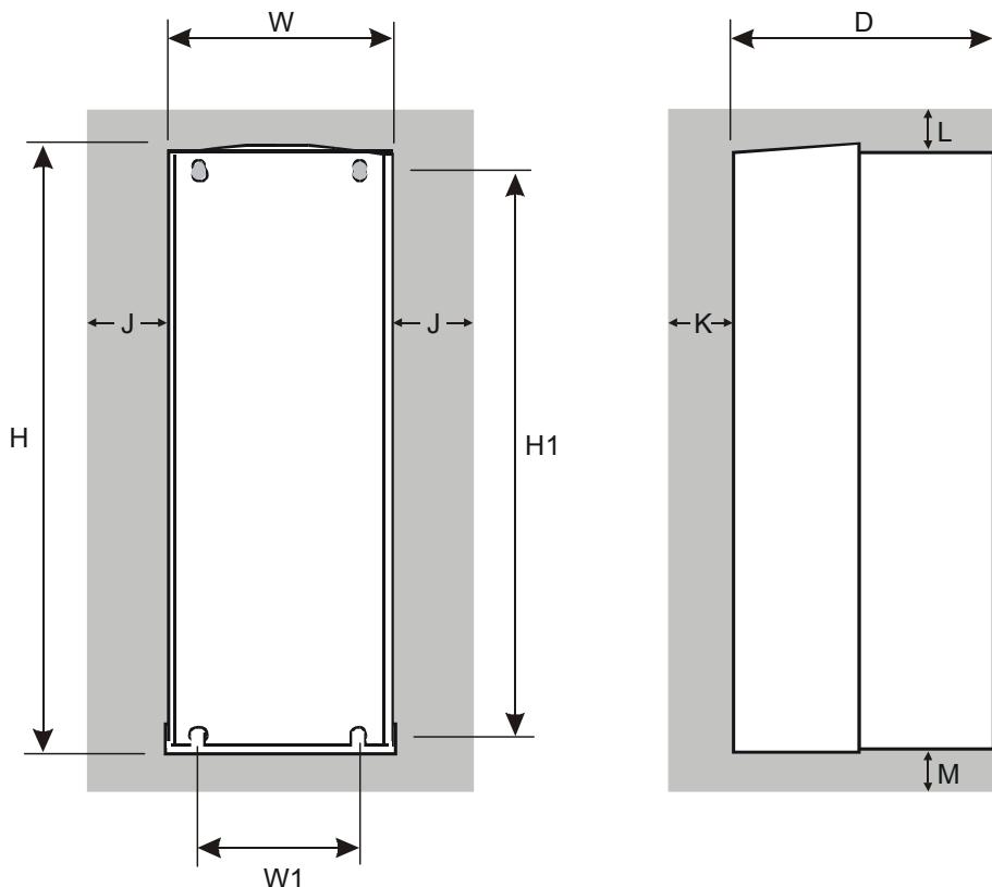
The units must be installed in a cubicle. Mount the drive using the keyholes and slots.
