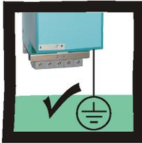
The unit must be **permanently earthed** due to the high earth leakage current.
