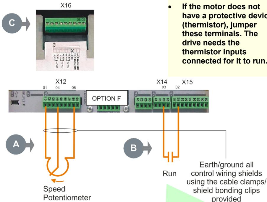
The control terminals will accept a single wire of size 1.5mm<sup>2</sup>/16AWG. For two wires per terminal, use smaller gauge wire such as 0.5mm<sup>2</sup>/22AWG.
