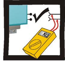
Disconnect the unit from circuits when doing high voltage resistance checks.
