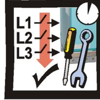
Before working on the unit, isolate the mains supply from terminals L1, L2 and L3 and wait 3 minutes.
