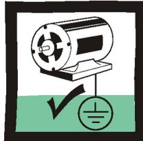
The drive motor must be connected to an appropriate safety earth.
